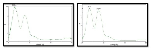
Fig. 2: Potassium dichromate and Sodium nitro prusside solution spectra.
